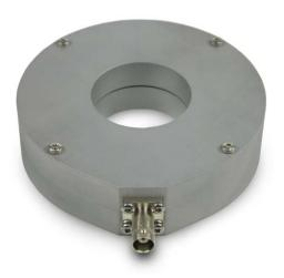
Current Monitoring probes may be used for RF current measurements with the advantage that there is no loading of the circuit, thus allowing normal operation of the DUT while the measurement is done. The CDG CMP-46 measures RF common mode currents (asymmetrical currents) of single conductors or bundles of conductors (the sum of currents considering the sign is of importance).
